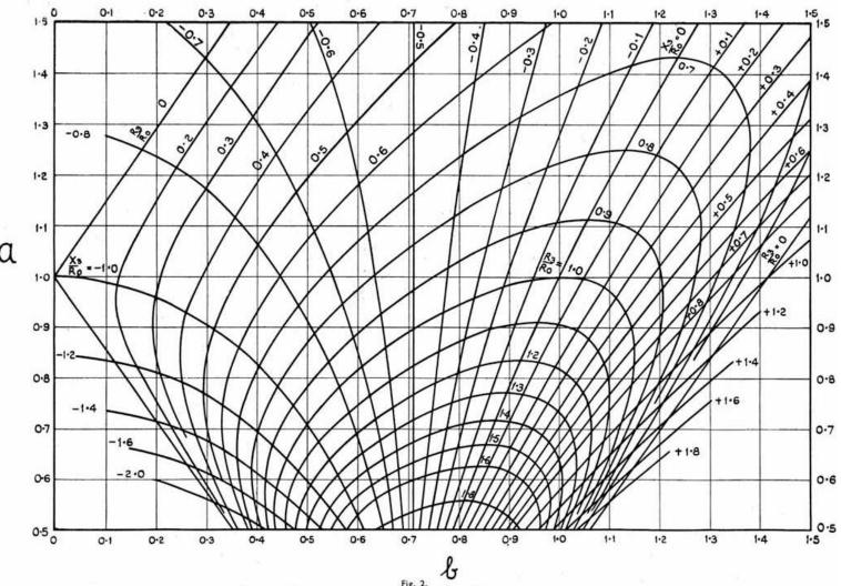
Chart to determine impedance of load, in terms of  $a = \frac{V_1}{V_3}$  and  $b = \frac{V_2}{V_3}$  Knowing a and b, the values of  $\frac{R_3}{R_0}$  and  $\frac{X_3}{R_0}$  are found from the chart. These values, multiplied by  $R_0$ , (70 ohms for the instrument described) give the resistance and reactance  $X_3$  of the load.
