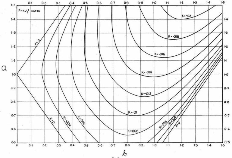
Fig. 3. Chart to determine power in load. Knowing a and b the value of K is found from the chart. Then  $P = K \times V_3^2$  watts.
