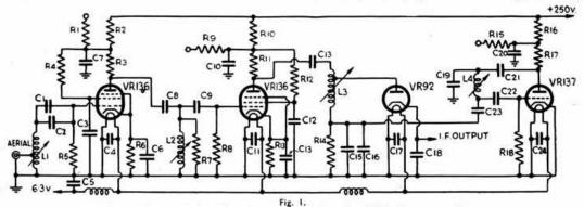
Circuit diagram of the R.F. unit as removed from the R3118. Component values:
