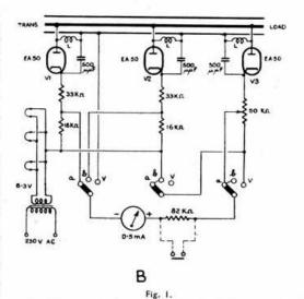
A. Simplified circuit. B. Actual circuit. All fixed resistors should be of the high stability type (Welwyn ½ watt or Erie Type 100). The potentiometer must be wire wound and as near to 50,000 ohms as possible. The dotted connections show the suggested addition of a push-button to short-circuit the series resistance for final balancing adjustment.
